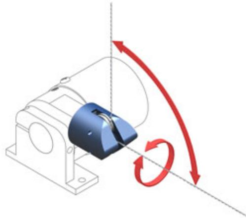
Figure 18 - The RoundAbout™ cable guide allows the displacement cable to exit the sensor at virtually any angle.
