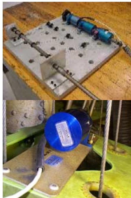
Figure 14 - DO-160D test fixture and on-aircraft installed sensor
